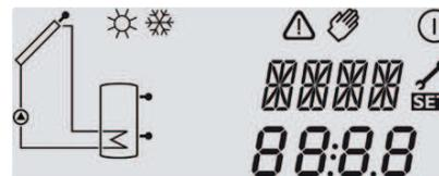
The System-Monitoring-Display consists of 3 blocks: channel display, tool bar and system screen.
