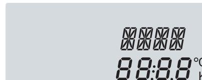
The channel display consists of 2 lines. The upper display line is an alphanumeric 16-segment display. In this line, mainly channel names and menu items are displayed. In the lower 16-segment display, values are displayed.
